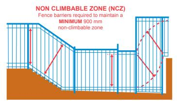
Where a barrier is sloping the measurements are perpendicular to the top of the barrier to maintain the integrity of the required NCZ and barrier height.
